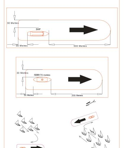
Be mindful of larger ships' bow flare. When closing any vessel, to prevent being overrun ensure you remain within sight of the Master / Officer of the Watch on the vessel's bridge. Beware of overhanging bows and other parts of ship that might obstruct this line of sight. This means that your vessel may disappear from sight inside 500m from the bows of very large ships.
